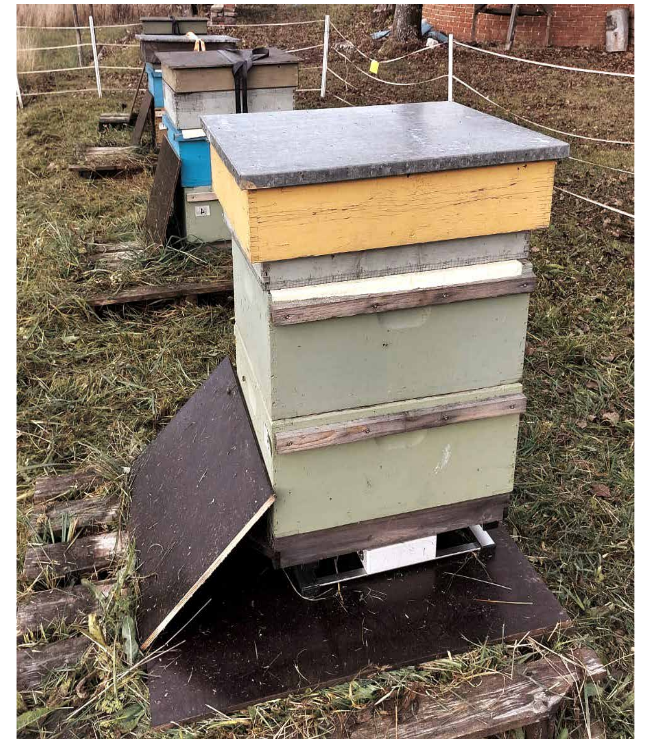
Fig.1. A combination of a hive and a hive scale forms one scale hive.
